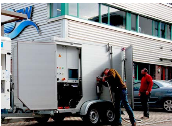
The new mobile measuring system for inspecting/approving H 2 filling stations. Photo: ZSW
