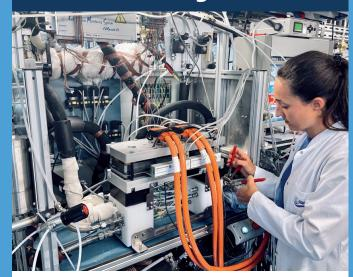
Already since 2001, the ZSW in Ulm has been operating a fuel cell test center with currently 35 fully automated test benches for professional 24/7-characterization of fuel cell stacks, systems and system components.
