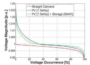
Figure 2.3 duration curve of the observed voltages for 57 households without PV, with PV and with storage.
