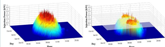
Figure 1.1 Profile Grid Injection Duration Curve without and with delayed charging.
