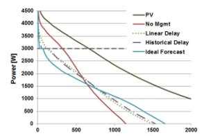
Figure 2.2 local duration curve for injected power [1] with delayed charging variants to reduce peak injection.
