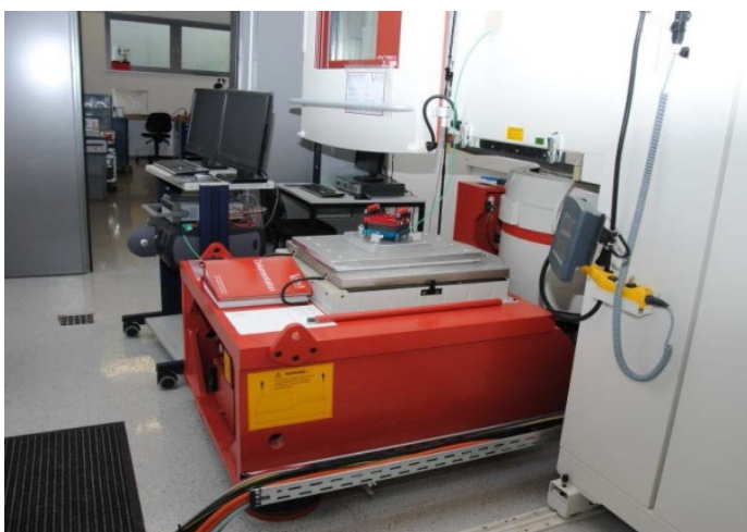
Vibration table with acceleration force of 20 kN, load up to 50 kg, possibility of thermal and electrical superposition
