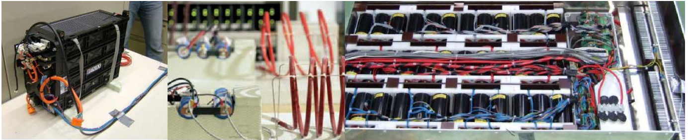
Li-Hybrid Module - Single cell measurements - 400V-Li-Hybrid System
