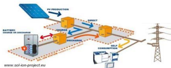
Figure 1: Sol-ion system with two DC/DC convertors towards PV generator and battery and one AC/DC convertor to connect to 235 V output line. The system is shown in two operation modes, connected to the grid and stand-alone.
