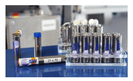
Battery prototypes produced by ZSW in 21700 format with aqueous-coated nickel-rich cathodes.
