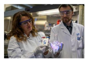
ZSW's RecycleMat team used reactivated anode and cathode materials to build pouch cells and power an LED light chain.
