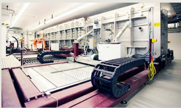
// The R2R web coater for CIGS deposition at ZSW
