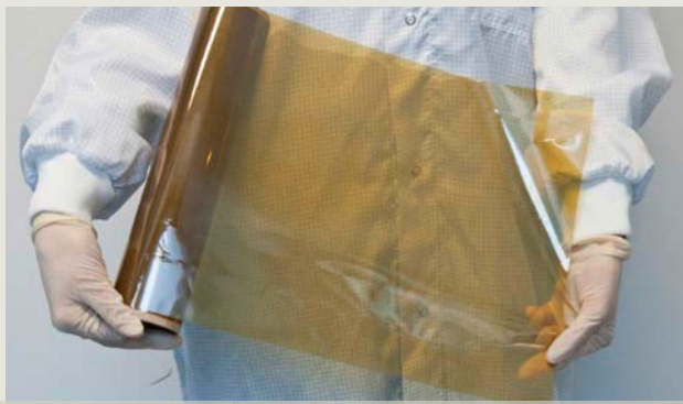
// Thin polyimide film used in ZSW web coater at low temperatures
