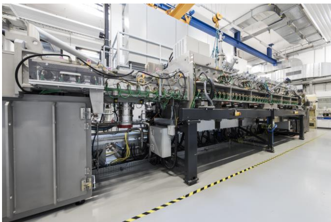
Production-like inline coating system at ZSW for development of absorbers for thin-film photovoltaics.
