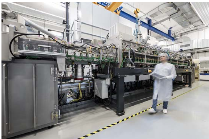
Lab plant for depositing the CIGS layer in a coevaporation process.
