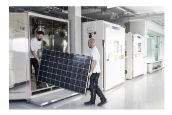
A look inside Solab, the ZSW module-testing laboratory where solar modules undergo the new heavy-duty trial to gauge their resistance to PID. Photo: Alexander Fischer / ZSW
