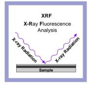
The sample is excited by x-ray beams with energies up to 50 keV. X-ray fluorescence radiation which is characteristic for each element is produced by the ionisation of inner atomic shells and subsequent transitions of electrons from higher energetic states into these ionised states.
