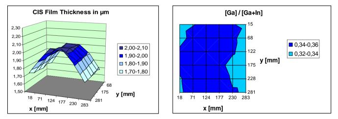
For quality control of our CIS modules we regularly perform linescans and mappings with XRF. The large information depth of XRF enables us to calculate from a single measurement the film thickness of the ZnO front contact, the CdS buffer layer, the CIS absorber, and the Mo back contact, as well as the CIS film composition. The thickness of the absorber and the Ga / [Ga+In] ratio of a 30 cm x 30 cm CIS modul are shown as examples in the figures.
