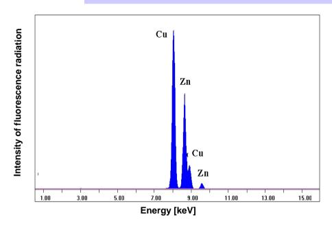
XRF spectrum of an unknown contact material. The analysis reveals that the material consists of 65 % Cu and 35 % Zn, thereby identifying it as a brass alloy.
