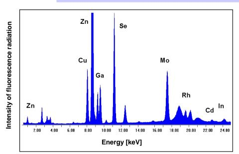
XRF survey spectrum from a CIS solar module. The Zn from the ZnO front contact, the Mo from the molybdenum back contact, and the Cu, In, Ga, and Se from the absorber are easily recognisable. The Cd peak is noticeably smaller since the CdS film is very thin. The peak integrals of the K-lines are used for quantification.
