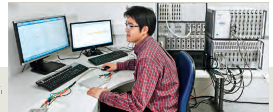
// Impedanzmessung an elektrochemischen Energiespeichern. // Measuring the impedance of electrochemical energy storage systems.
