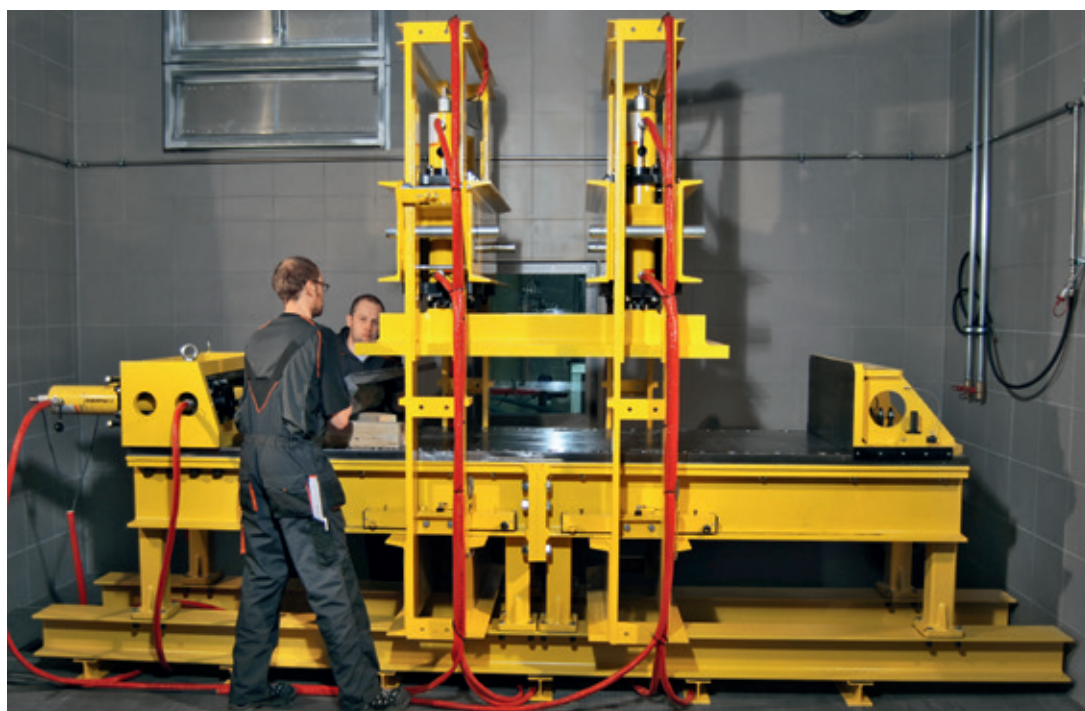
Test bunker equipped with a press for 100-tonne crush tests and video surveillance.
