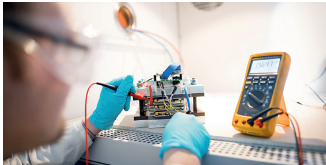
Characterising battery cells via impedance spectroscopy.
