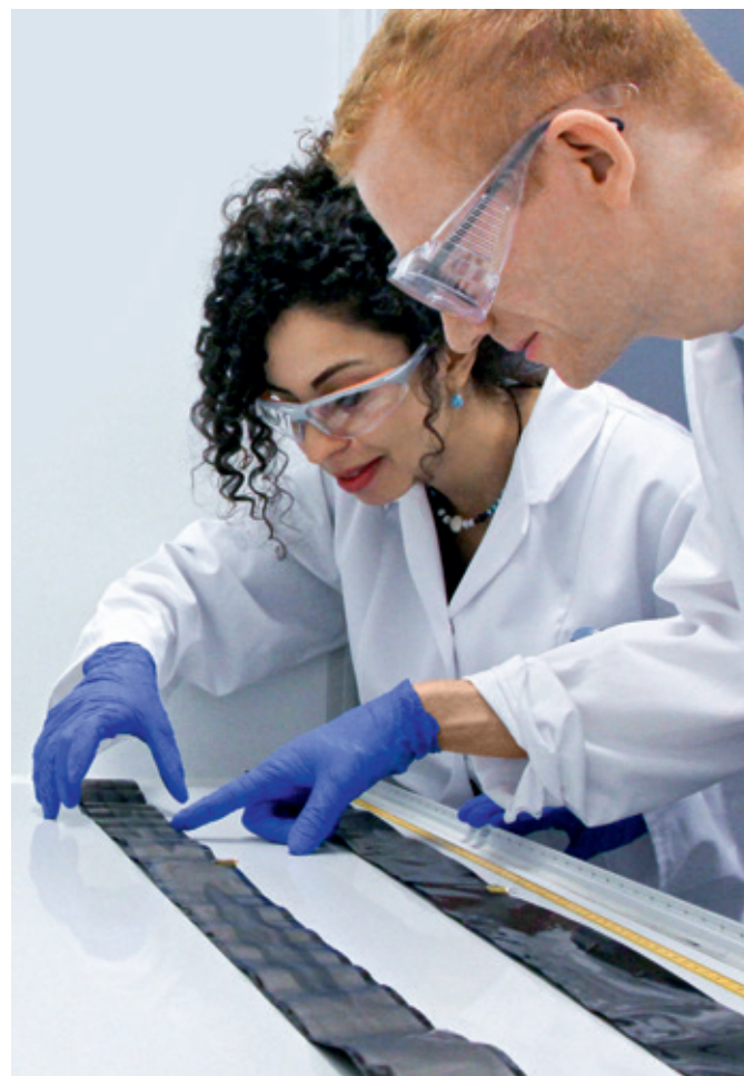
Visual inspection and sampling of electrode strips that were washed and rolled out after opening the cell.
