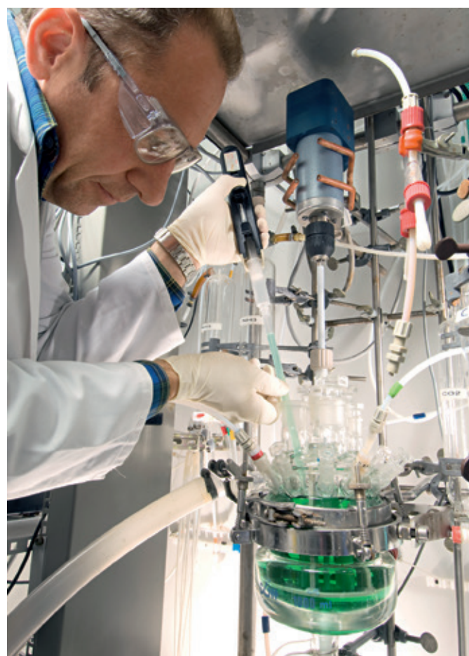
Synthesis reactor for manufacturing active material on a kilogramme scale.
