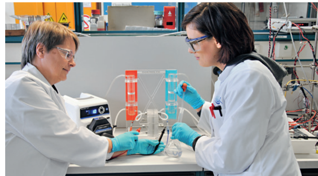
Alkaline electrolysis at atmospheric pressure in a lab cell.
