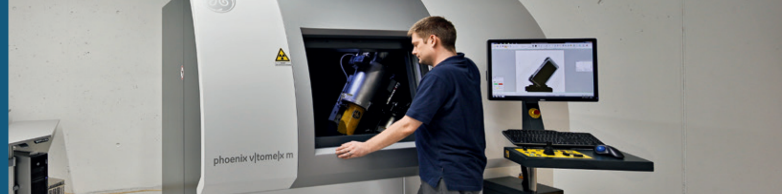
3D CT for non-destructive Li-ion cell testing.
