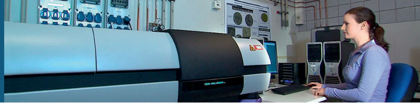
Using microcomputer tomography (μ-CT) to characterize porous fuel cell components ex-situ.
