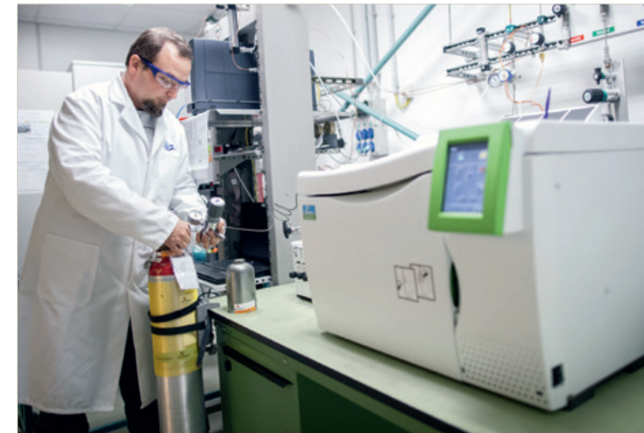
Analytical laboratory for determining hydrogen samples quality according SAE J2719/ ISO 14687-2.
