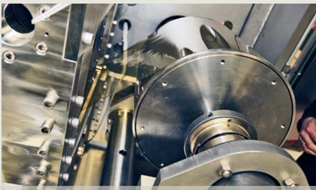
// Winding unit of the R2R web coater at ZSW
