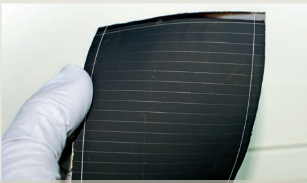
// Monolithically integrated mini-module on insulated, stainless steel substrate with an efficiency of > 10 %
