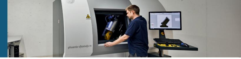
3D CT for non-destructive Li-ion cell testing.
