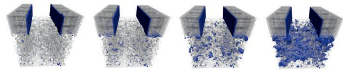
A Monte Carlo simulation showing the effect of varying amounts of PTFE on water distribution in the GDL
