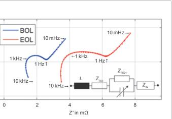
Electrochemical impedance spectra of a cell at the beginning (BoL) and end of life (EoL).
