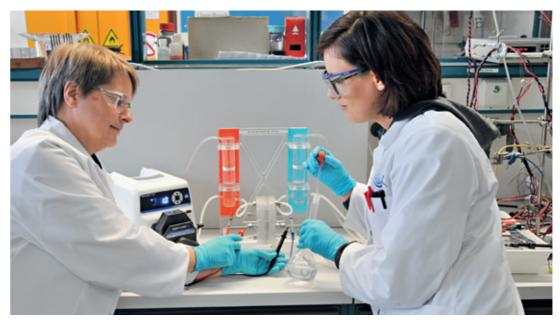
Alkaline electrolysis at atmospheric pressure in a lab cell.
