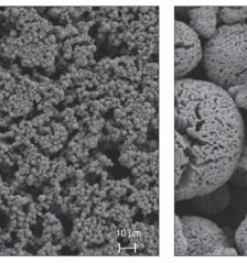
SEM images of surface nickel electrodes showing a coating of nanostructured nickel particles on nickel foil.
