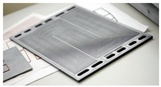
Bipolar plate with an optimised gas manifold structure.
