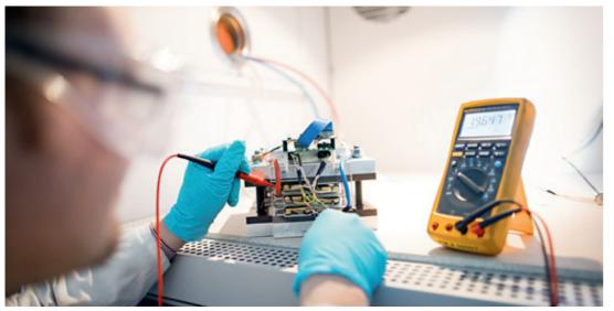
Characterising battery cells via impedance spectroscopy.
