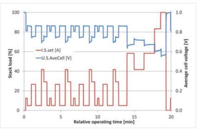
Fuel Cell Dynamic Load Cycle (FC-DLC), a harmonised life-cycle test developed by ZSW.
