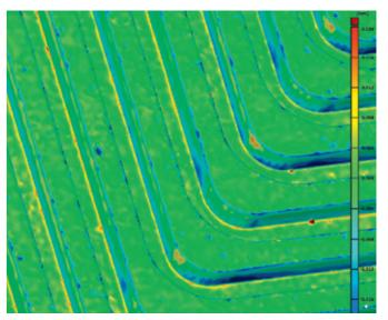
CAD data are compared with measured 3D data to verify bipolar plates' quality.
