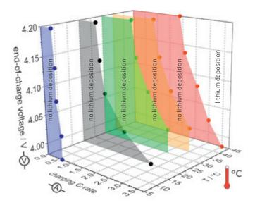
Operating parameters' influence on Li deposition in pouch cells. Source: ZSW/T. Waldmann et al., J. Electrochem. Soc., 163, A1232 (2016).
