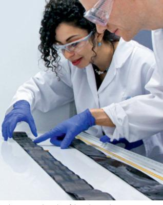
Visual inspection and sampling of electrode strips that were washed and rolled out after opening the cell.
