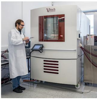
Temperature chamber for electric battery tests.
