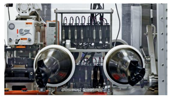
Lab device for closing and filling 18650 cells.
