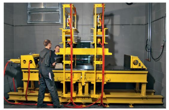
Test bunker equipped with a press for 100-tonne crush tests and video surveillance
