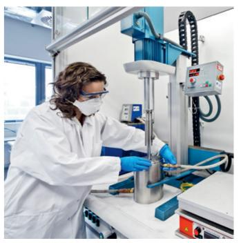
Lab mixer for electrode slurries.
