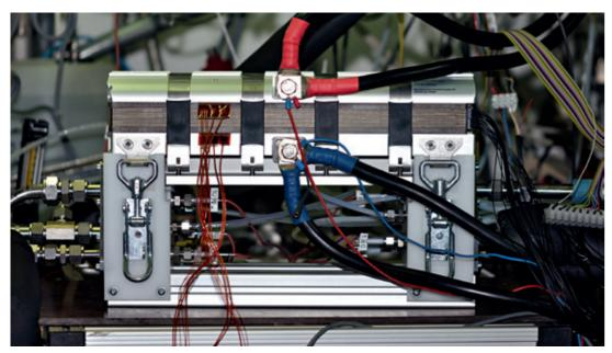
A short stack of a vehicular high-performance fuel cell on the test bench.
