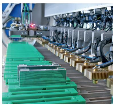
Pre-formation system for wound prismatic cells (PHEV-1 format).
