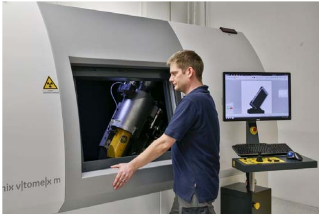
The new dual-source X-ray scanner at ZSW. Photo: ZSW/Duckek
