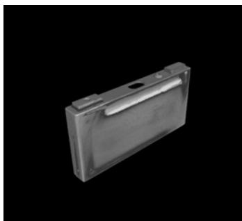
3D-CT image of a Lithium-ion battery for electric cars (PHEV-1 cell design). Photo: ZSW
