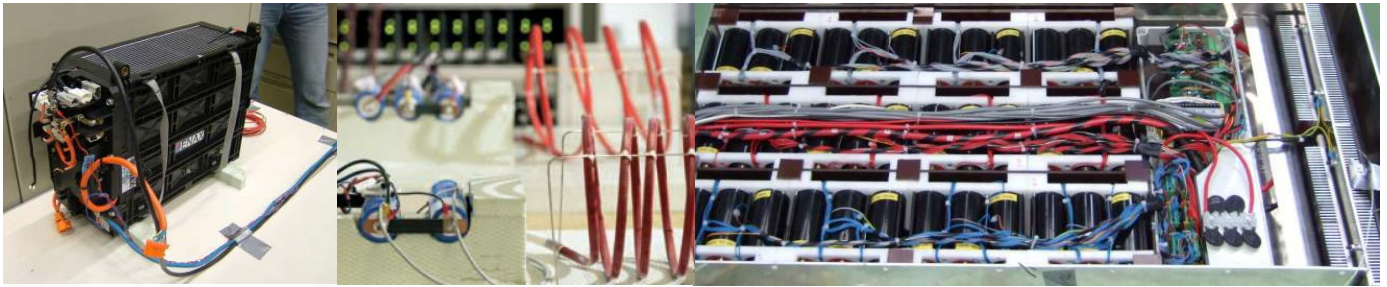
Li-Hybrid Module - Single cell measurements - 400V-Li-Hybrid System
