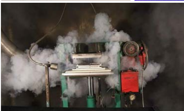
Cell with not controlled dissipation of power
