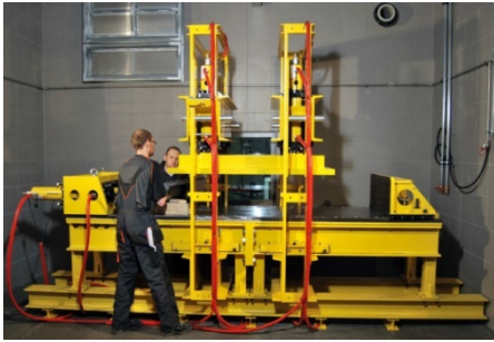
Test bunker with mechanical press with 100 tons max. force and video observation
