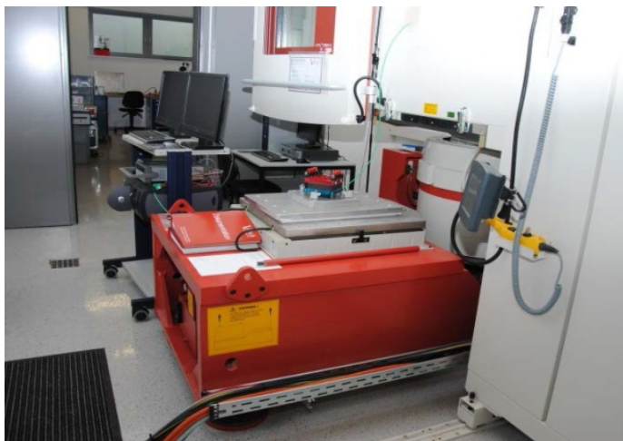
Vibration table with a acceleration force of 20 kN for load up to 50kg, possibility of thermal and electrical superposition
