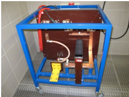
Short circuit equipment, max. current 15 kA / Oven with 1500 l volume
